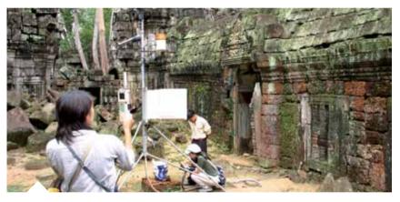
Measurement of the hardness of the stone and its microflora in a microclimate
