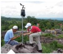
Installation of a meteorological station in the Kulen Mountain
